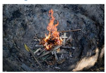
Start a small fire in the middle of the pit by using small pieces of chopped bamboo, paper etc. Keep adding material, until the fire is filling up almost the whole bottom of the pit. Now you can add the coconut husks around the fire by placing in such a way, that airflows crawling downwards the side are interrupted.
